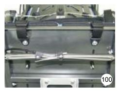
Thread the attachment straps of the groin strap between seat and back padding, wrap them around the back of the seat edge and attach with rectangle-rings, the screws and the washers under the seat plate.
