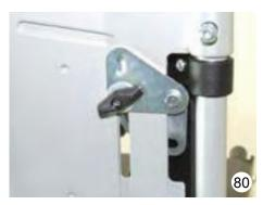
The triangular pad guiding gets plugged from the back side The stamping in the pad guiding must be positioned into the long hole.
