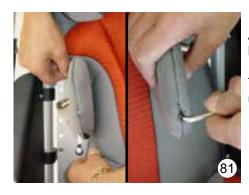
After reaching the desired position and tightening the wing nuts the back upholstery is pushed underneath the trunk pads.
