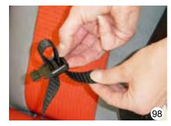
Position the groin strap with the quick-release buckles on the thigh belts pointing downwards on the seat surface.
