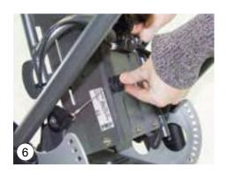
• Pull the seat unit on the backrest to the back (7) until the mechanism of the tilt function engages hearable in the first position.
