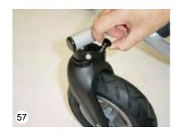
After loosening the clamping screw the track can be adjusted with engaged swivel lock.
