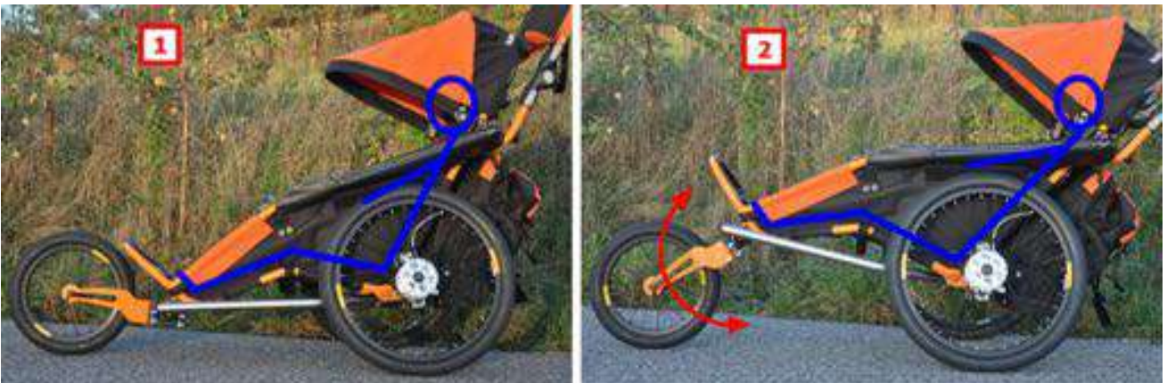
Figure 19 – stroller seat tilt: 1 – sitting position; 2 – lying position
