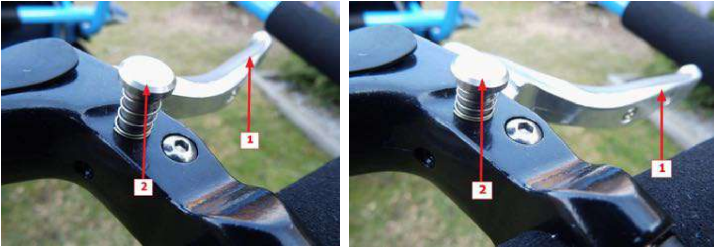
Figure 26: A – parking brake deactivated; B – parking brake activated
